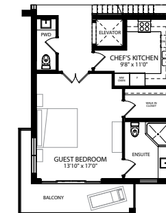
PARTIAL 2ND FLOOR PLAN BEACH FRONT EXT/INT END UNIT OPTIONAL CHEF'S KITCHEN
